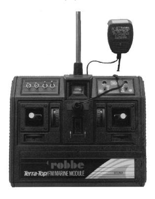
**Caution:** Do not overcharge the batteries as this could cause permanent damage to the transmitter batteries. (Doubling the normal charging time is the type of over charging that is meant here, and the battery getting hot.) When the battery level needle goes in the red, the robot should be turned off because the robot could act erratic without the transmitter signal.
